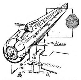
Fig. 1. The finished fuselage block, showing cut-out for lower 'plane, octagonal cross-section and threads representing cowling joints
