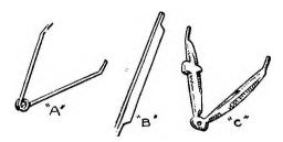
Fig. 2.—Two varieties of struts. The plain wire vee ("A") and the sheet metal type ("B" and "C"). "B" is an interplane strut before streamlining, "C" is the finished left-hand undercarriage vee with petrol pump
